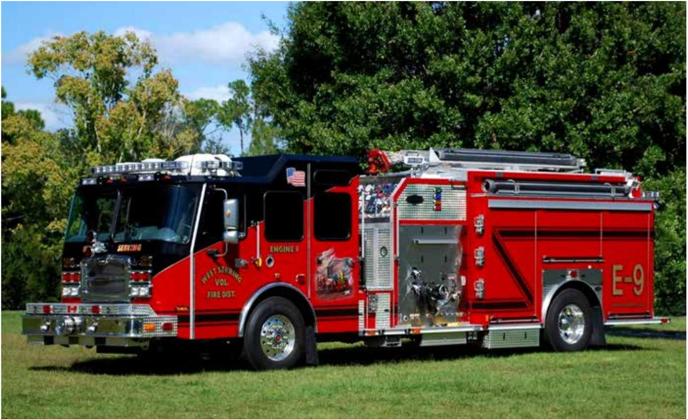
E-ONE® pumpers are the most versatile, durable pumpers on the market. Offering both aluminum and stainless steel bodies, tank sizes up to 1530 gallons and available on either custom or commercial chassis, E-ONE pumpers will meet your unique performance and budget needs. Safety is never secondary at E-ONE. Our stepping surfaces exceed NFPA standards and our plumbing and electrical systems undergo extensive third-party testing.
