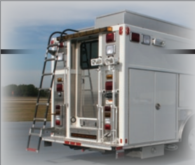
Rear entry door, roof top access ladder.
