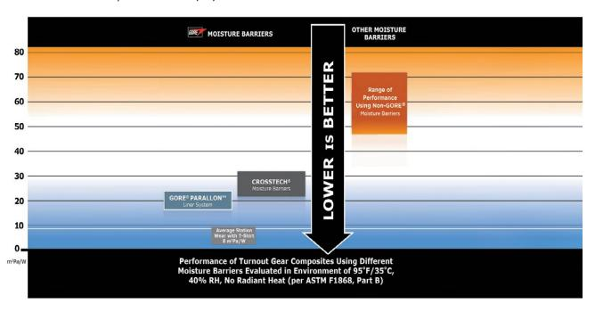
When tested using the ASTM F1868, Part B method, GORE\* barrier technologies created less resisitance to evaporative sweat transfer, enabling higher breathability when evauated in the same outer shell and thermal liner combinations.
