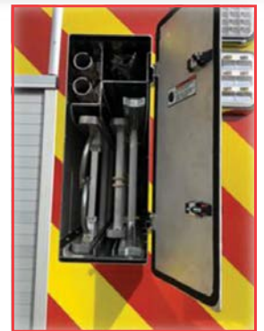
24-ft 2-section; 14-ft roof; attic; and (2) pike poles stored in the body.
