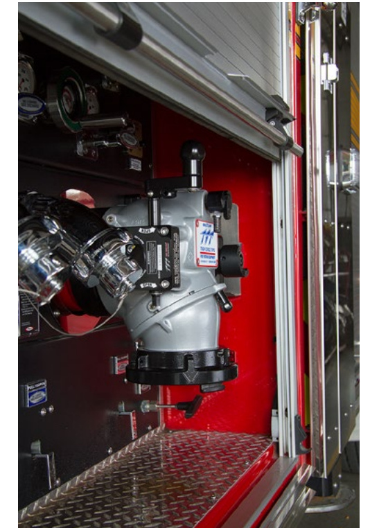
Low Profile BIV versions for tight pump panels.
